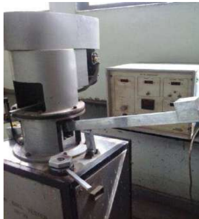
Figure 1. The Four Ball Extreme Pressure Oil Testing Machine.
